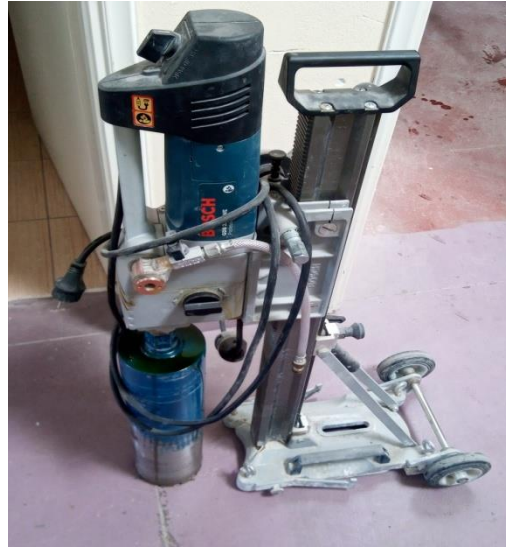
Apparatus for concrete core extraction.
