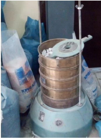
Sieving apparatus for aggregates.
