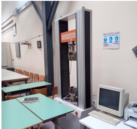
Tension/compression machine for testing rebars.
