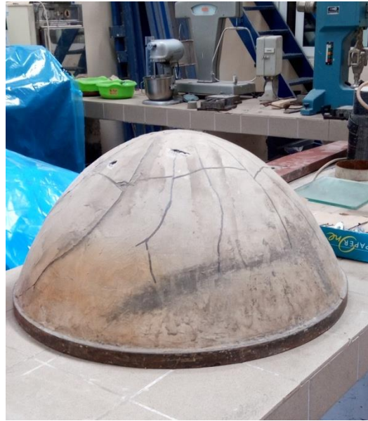
Fractured cement mortar dome.
