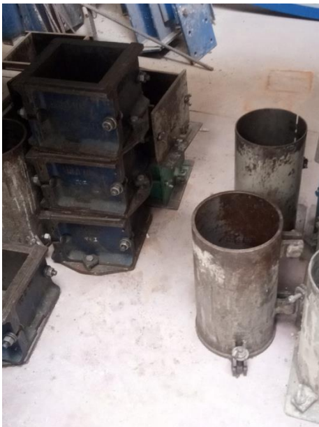
Cubic and cylindrical steel moulds for concrete.
