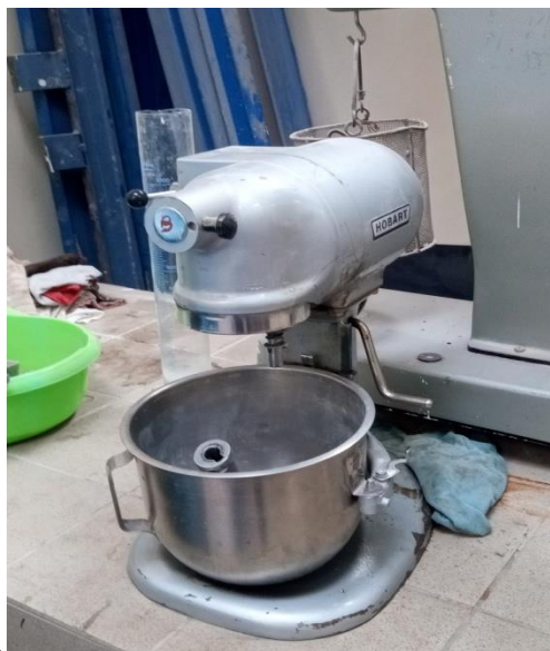
Mixer for production of cement mortar.
