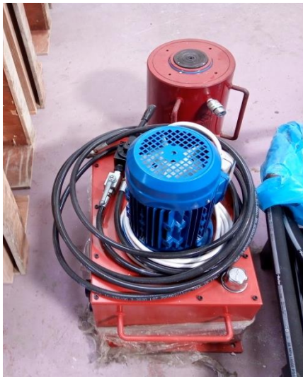
Piston for static loading of 100 kN capacity.
