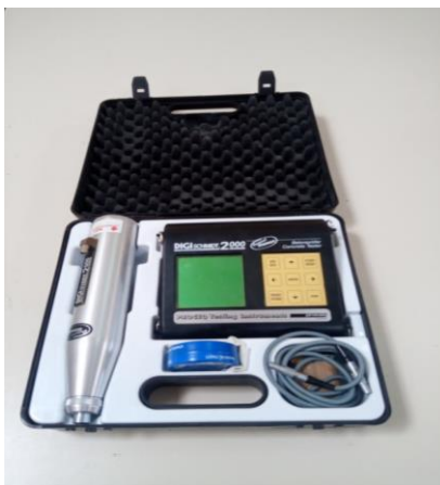
Ultrasonic emission apparatus for concrete strength estimation.
