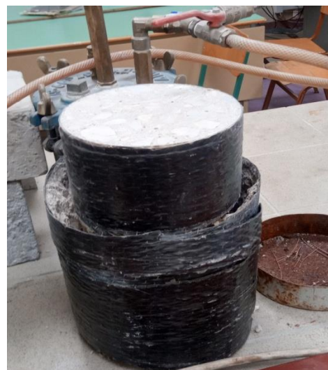
Failure of strengthened concrete cylinders by CFRP.
