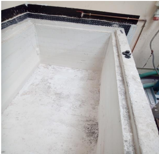
Water vat for curing of concrete specimens.
