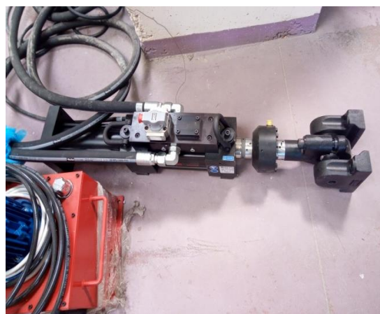
Piston for seismic loading of 100 kN capacity.
