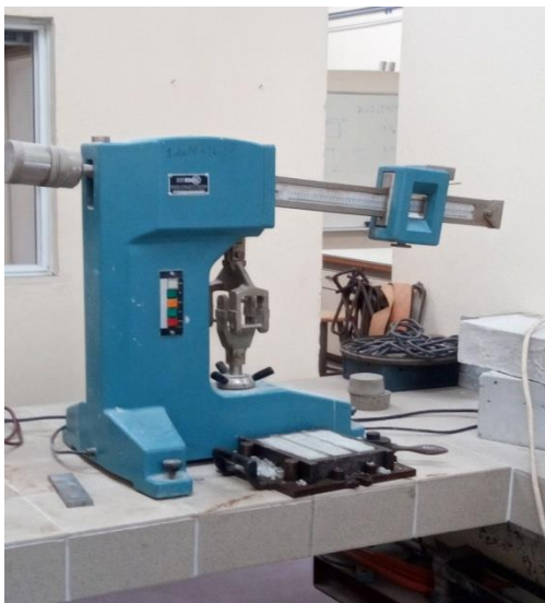
Bending apparatus for cement mortar specimens.
