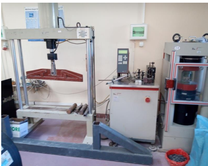
Bending machine for beams.
