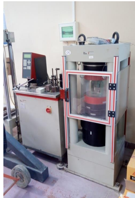
Compression machine for concrete specimens.
