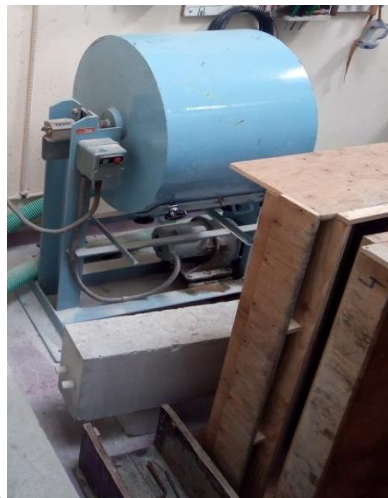
Los Angeles machine for friction test of aggregates.
