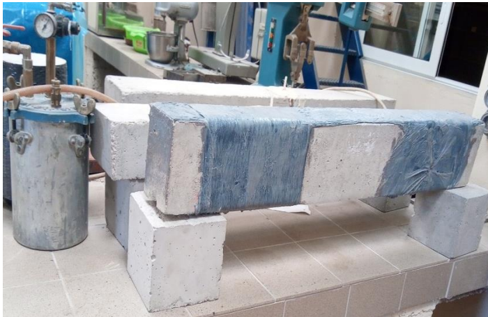
Strengthened RC beam by CFRP.
