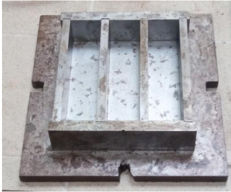
Moulds for casting cement mortar specimens.
